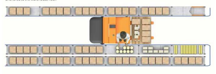
Each model of machine needs its own type of guide rail and a distinct aisle width. The aisle width is defined by the distance between the guide rails and the distance between the load levels.
